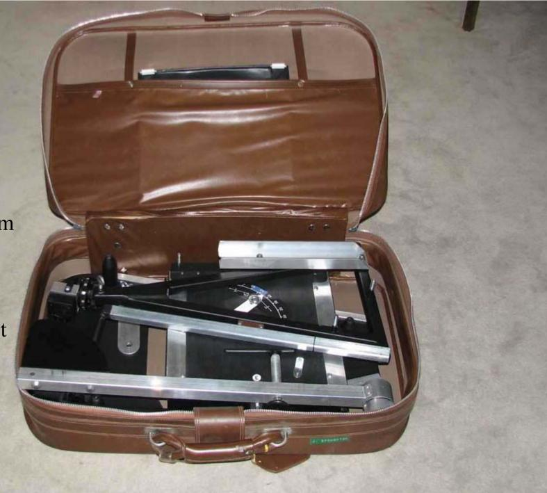
The Suitcase Telescope set up for observing (except for the cameras). 3 can be set up ready to go and put on the back seat area of an ordinary car; more could be put in the trunk.
